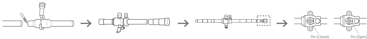
1. Cut the inlet side of the connector, and weld the pipe
