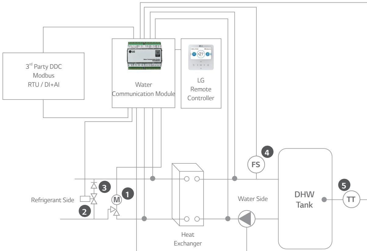
\* 3<sup>rd</sup> party solenoid, non-return valve, heat exchanger, flow switch and DHW temperature transmitter (Optional) must be purchased separately. (Field supplied items)
