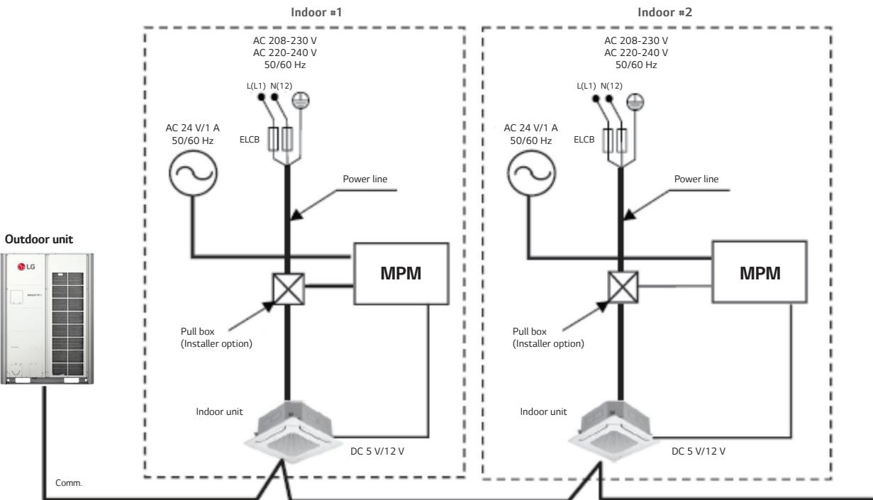
※ When Multi-tenant Power Module is adopted, CN-EXT must be used for it. Instead of being used CN-EXT, PDRYCB000 (220Vac input) / PDRYCB100 (24Vac input) Module are being used for Single contact.
