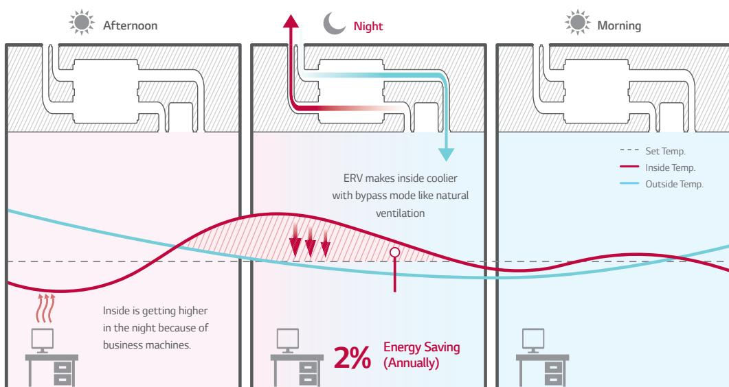
※ This function is operated with 'Night Time Free Cooling' on remote controller (with MULTIV only)
