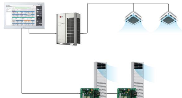
\* The Commercial Air purifier must additionally install PI485(PHNFP14A0).
