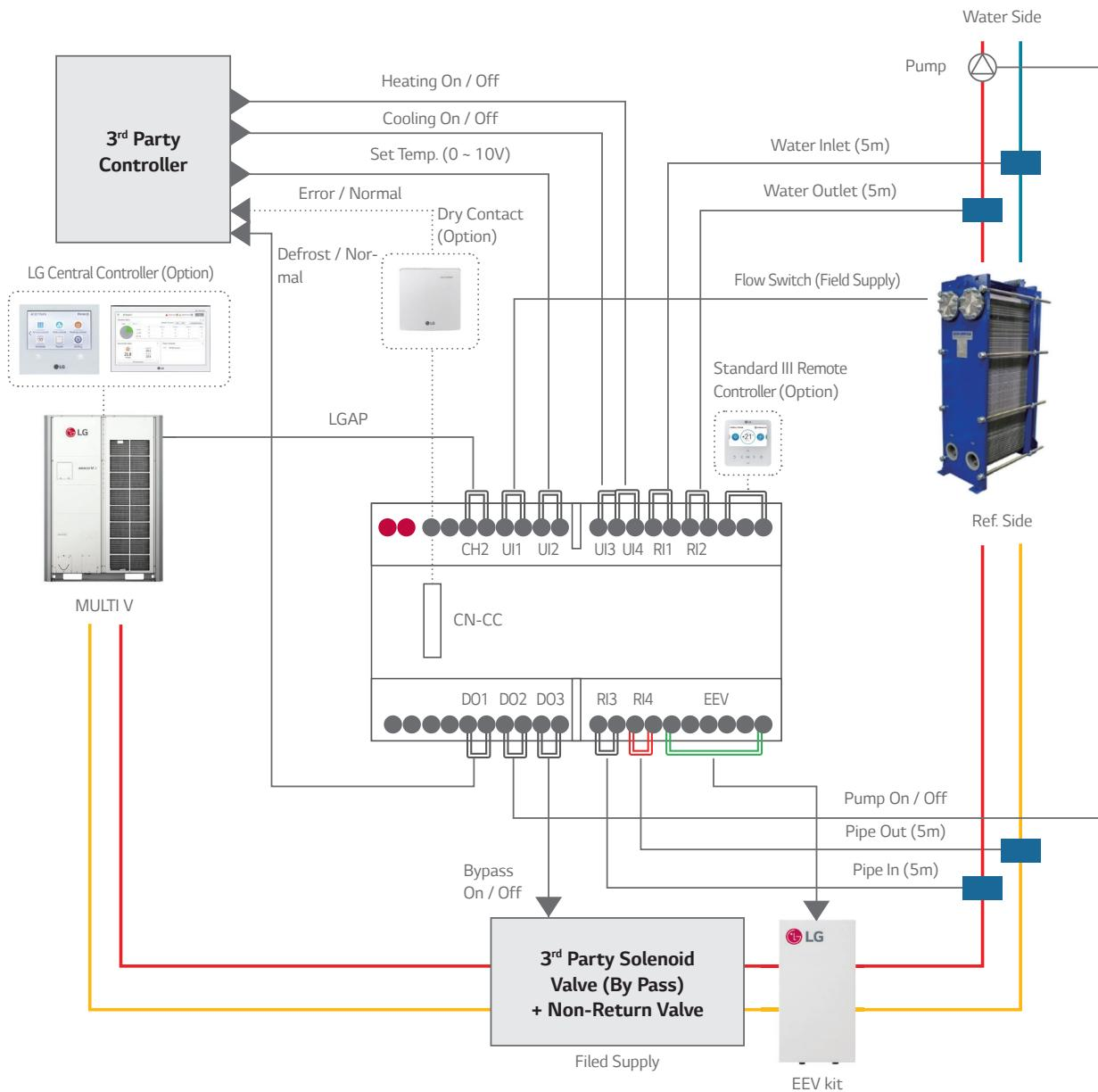
**Installation Scene with Modbus / LG Control (Optional) Connection**
