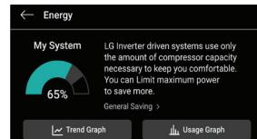
The Energy Navigation provides system operation trend per day. Running time and power consumption is also provided compared to last year by week, month and year.
