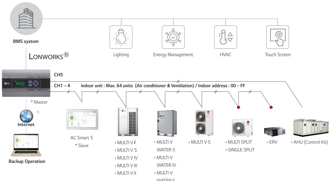
1) Assignment of public IP address is required to access central controller through internet.
