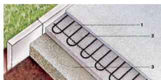
1 = béton 2 = tapis chauffant 3 = support
