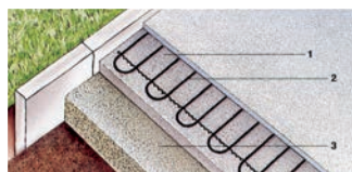
1 = béton 2 = tapis chauffant 3 = support
